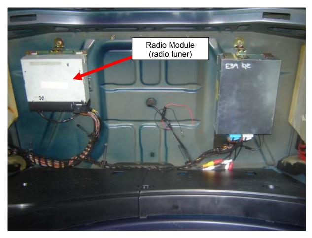
Unbolt the radio - 1 x nut, at bottom of radio module - and slide out of bracket
