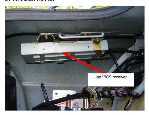
The VICS receiver is powered and connected to the Japanese nav unit directly – so when you remove the Jap nav unit, you will see the cable loom that goes from the nav to the VICS receiver. Remove and discard this loom at the same time you remove the VICS receiver.
