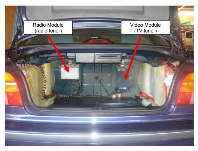
If you look carefully you will see the author has a (temporary) AV-in connection plugged in to the video module. This is my iPod connection to play movies on the AV in of the TV. After I took this photo I ran permanent AV cables to above the glove box.
